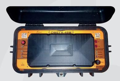
Resistivity instrument measures amplitude parameters of output current of the transmitter, electrical potential difference between measuring electrodes (apparent resistivity), time parameters of chargeability (apparent chargeability) determined on voltage decay curve at measuring electrodes after switching off the current.
