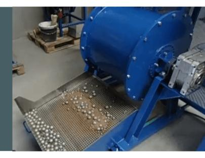
The most common test method used to indicate aggregate toughness and abrasion characteristics.
