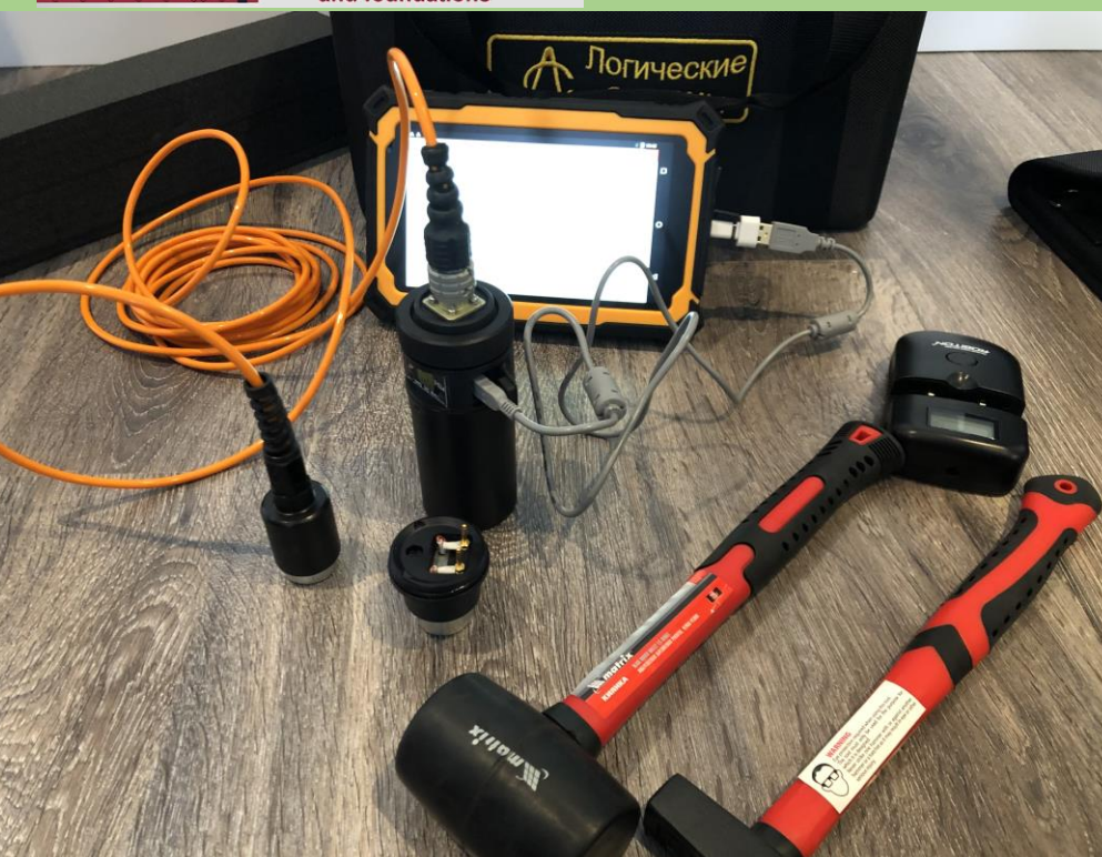
For inspection piles and foundations
